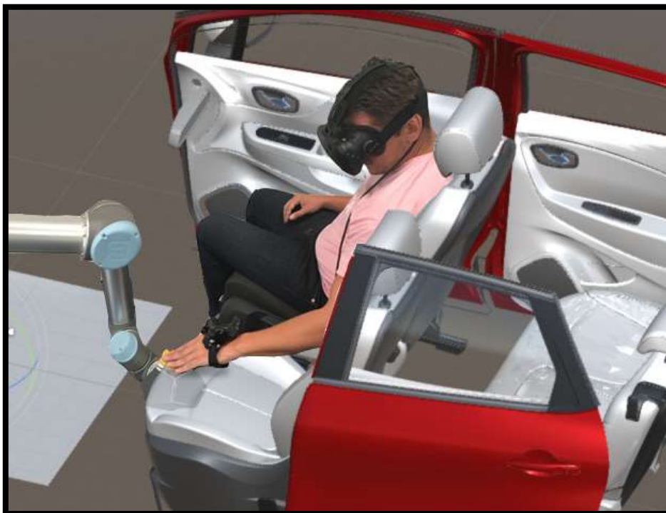
Figure 1. Use of an ETHD to touch the material of a virtual seat.
